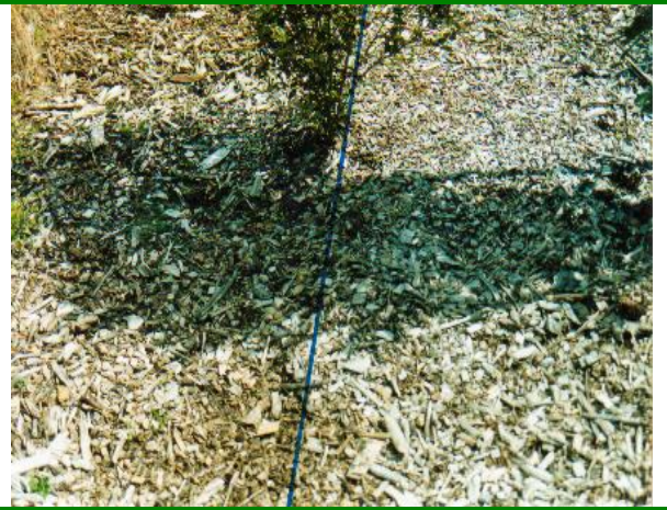
Right side – EcoCover consolidates bark Left side – Bark over plastic causes slippage
